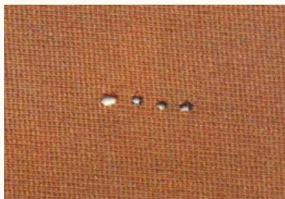
Damaged meshes of knitted fabrics by needle
