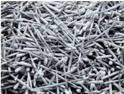
This is a process of freezing needles at about minus 100°C temperature which transforms the remaining austenite of the needle structure into martensite and furnishes the best limit of elasticity and increases the toughness after the tempering operation.
